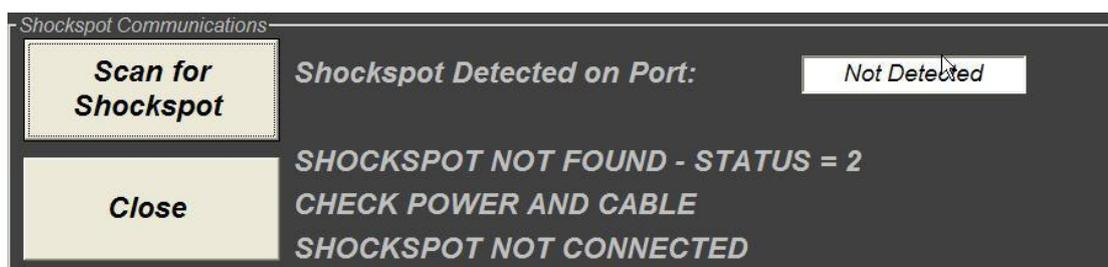
If you get this message when you click the connect button the most likely problem is that the driver is not installed for the Shockspot communication hardware. The drivers for Windows 10, 11 are available from this link: [www.shockspot.net/shockspot-software/Shockspot\\_Driver\\_v2.12.6.4.exe](http://www.shockspot.net/shockspot-software/Shockspot_Driver_v2.12.6.4.exe).
